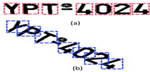
Fig. 5. Change of bounding box sizes of LP symbols due to rotation:
